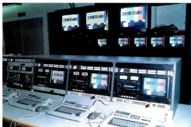
NOJC (Japan Pool) monitoring room using compact DVCPRO VTRs (AJ-D-230) IBC.
